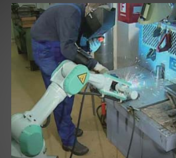
IPA : Direct Teaching Welding Robot called Rob@Work
