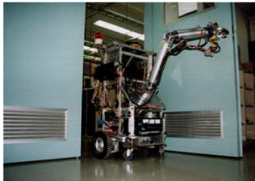
Autonomous Navigation with Door Opening/Closing (Yamabico-ten, 1998)
