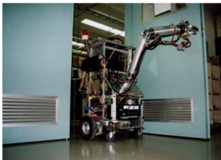
Autonomous Navigation with Door Opening/Closing (Yamabico-ten, 1998)
